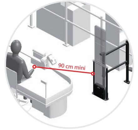
Leave at least **90 cm** between an EAS gate and the checkout scanner.
