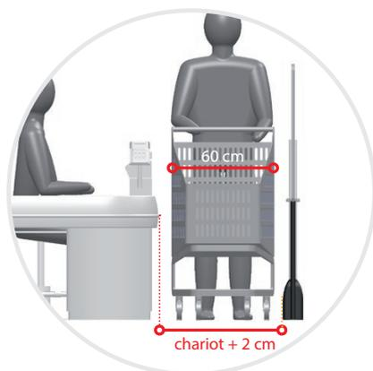
Position the security gate to clear a passage for the trolley
