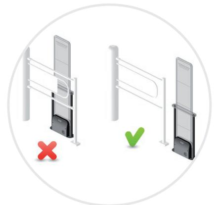
Position the antenna in line with the guidance gates.
