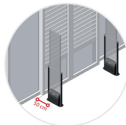
Leave **50 cm** between the gates and the automatic door or metal shutter.
